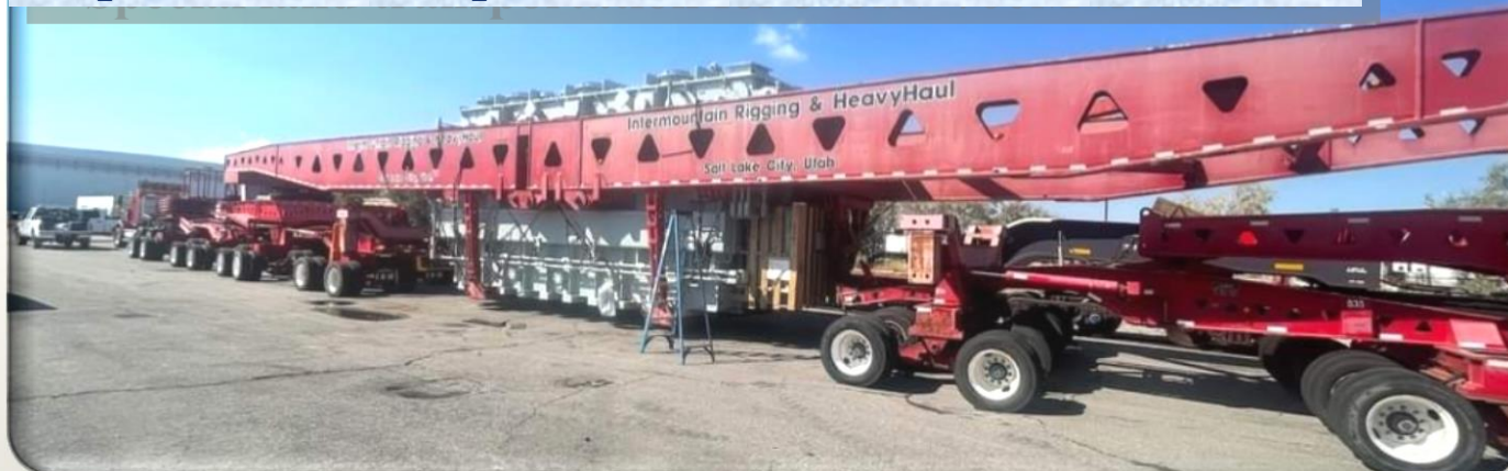
Special land transportation for 345kV 700MVA in USA
